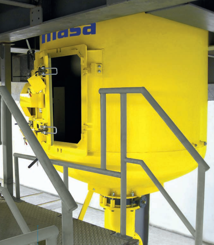
Fig 4: Lateral maintenance access to the high-performance mixer.
