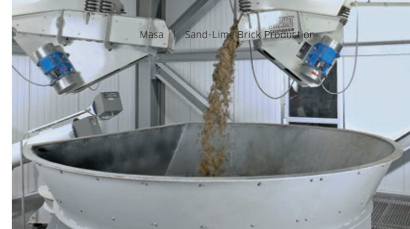
Component for the precise dosing of sand.
