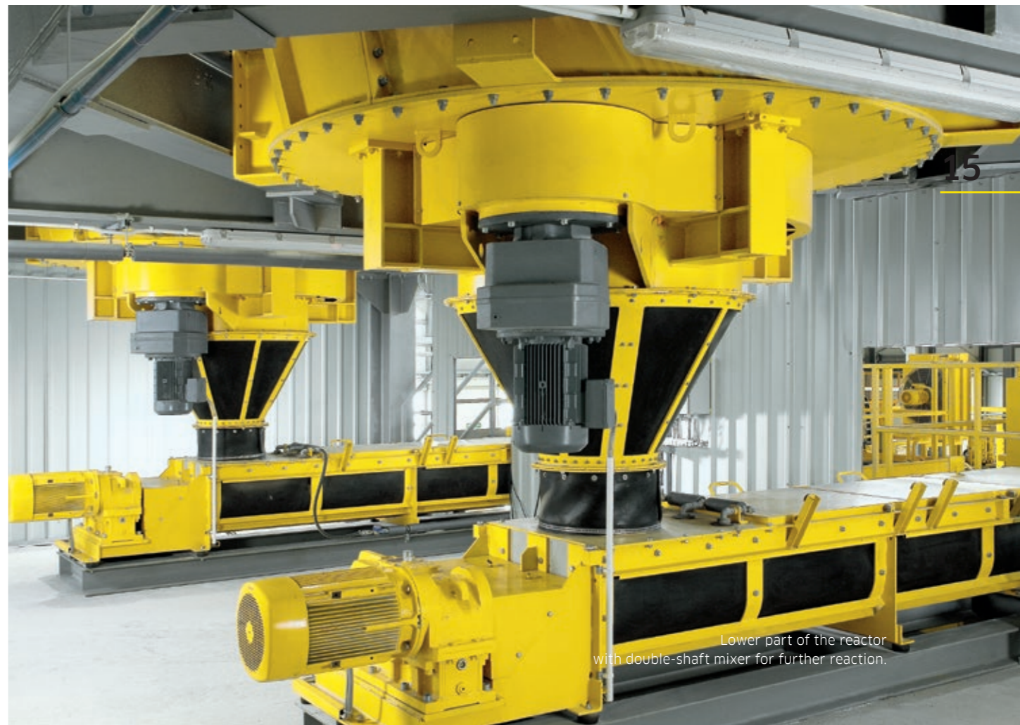
Intensive mixer for a homogeneous basic product.
