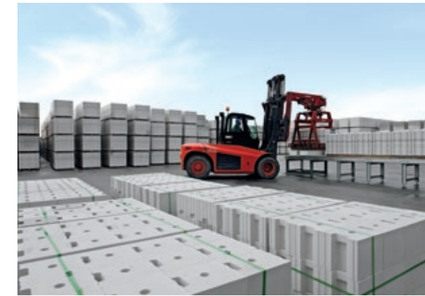
Removal of the strapped bricks
