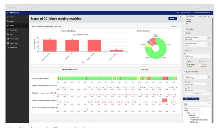
All machine data can be filtered and analysed with the Masa Service Cloud: Most frequent alarms, statistical and graphical distribution of states and state histories.
